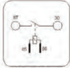
1A wiring Standard coil
